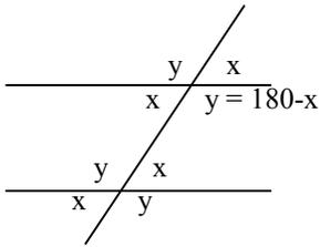
Visualize placing parallel lines on top of each other. All Xs and Ys are equal. Given any one angle, all others can be found.
